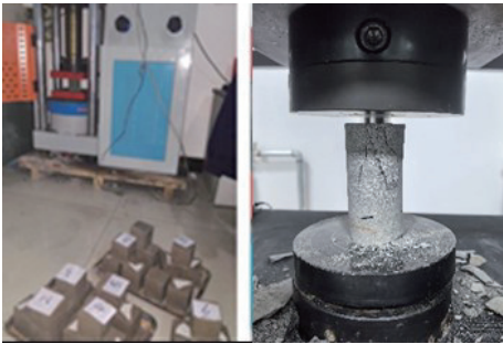
图 8 抗压强度测试试验 Fig.8 Compressive strength test
