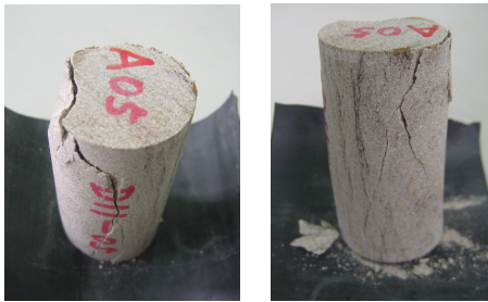
图 1 砂岩试样破坏图 Fig.1 Destruction of sandstone samples
